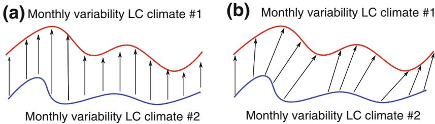
Fig. 1 Two ways of calculating distance between time series: **a** Euclidean distance and **b** DTW
